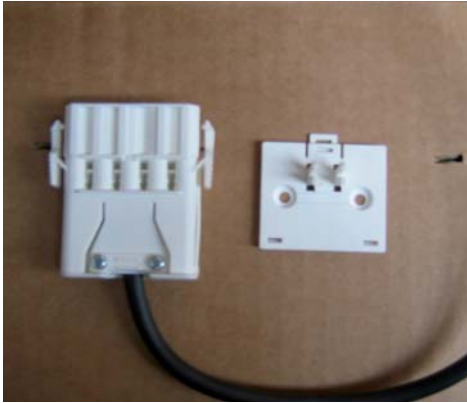
Remove the bracket from the male connector.
