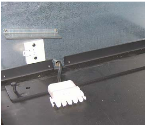
Fit the cable with female connector for ES 904 through the hole in the cassette.
